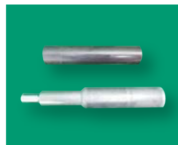
Power transmission shaft (top: material, bottom: finished product)
